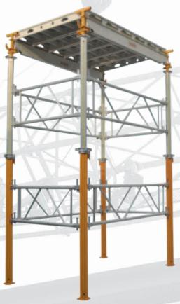
▲ Leader Aluminium Shoring & Slab Formwork System can be braced with frames to be used as slab tables or shoring towers for various height. In combination with frames to achieve essential stability. The Aluminium Shoring could withhold up to 90KN thus ensure safety and rigidity while reduce the prop consumption and cut cost effectively.
